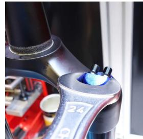
When tightening, ensure that the socket does not damage the fork crown.
